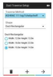
After pressing + to add a new duct size, you are brought to the **Flow Setup** page. To change the dimensions, use the arrow keys to navigate between Width and Height then press - to begin editing the numbers by using the arrow keys. Press  $\checkmark$  to save the new duct size.
