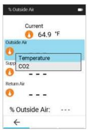
The **Percent Outside Air** feature offers the choice between using Temperature or  $CO_2$  for the Percent Outside Air study if a probe that supports either  $CO_2$  or Temperature is plugged in.
